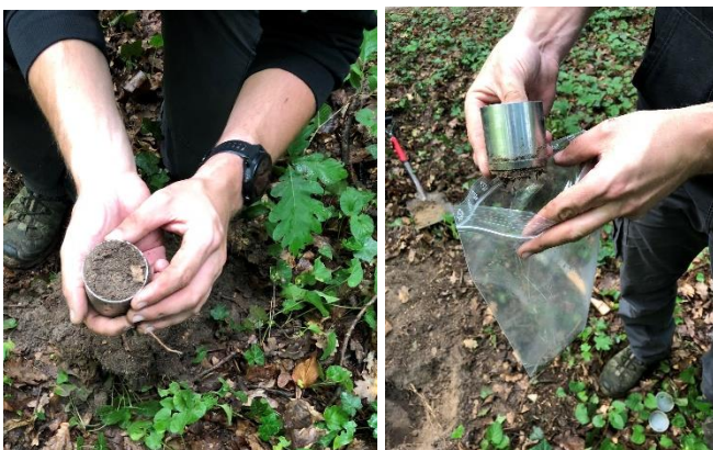
Figure 6.: The excavation of the ring and bagging
