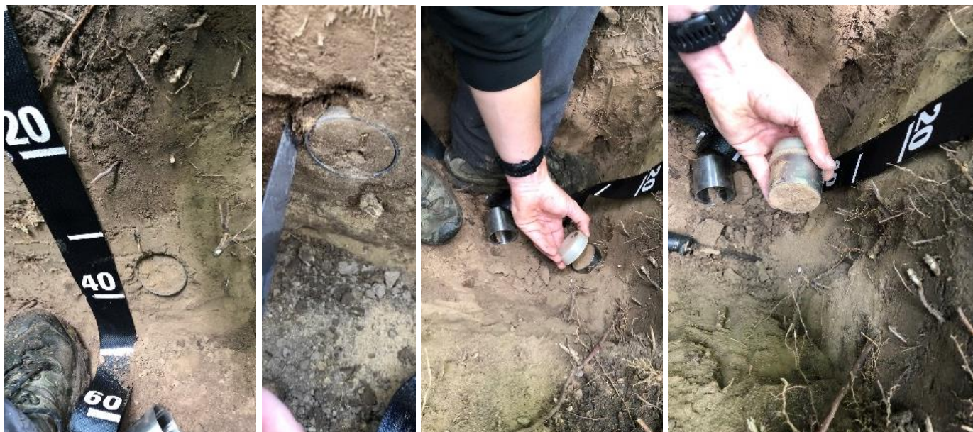
Figure 10.: Hammering the metallic ring into the soil, and the excavation
