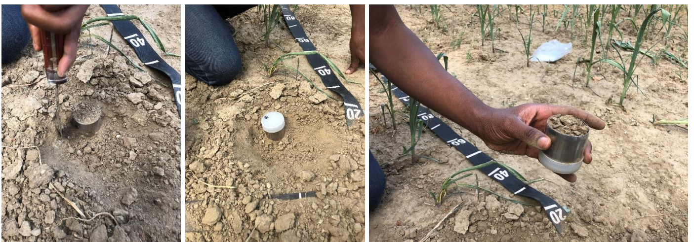
Figure 7. The extraction and excavation of the ring in case when the soil surface if compacted or too loose to be able to extract a clump
