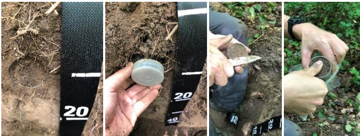
Figure 12.: Taking the undisturbed topsoil sample.
