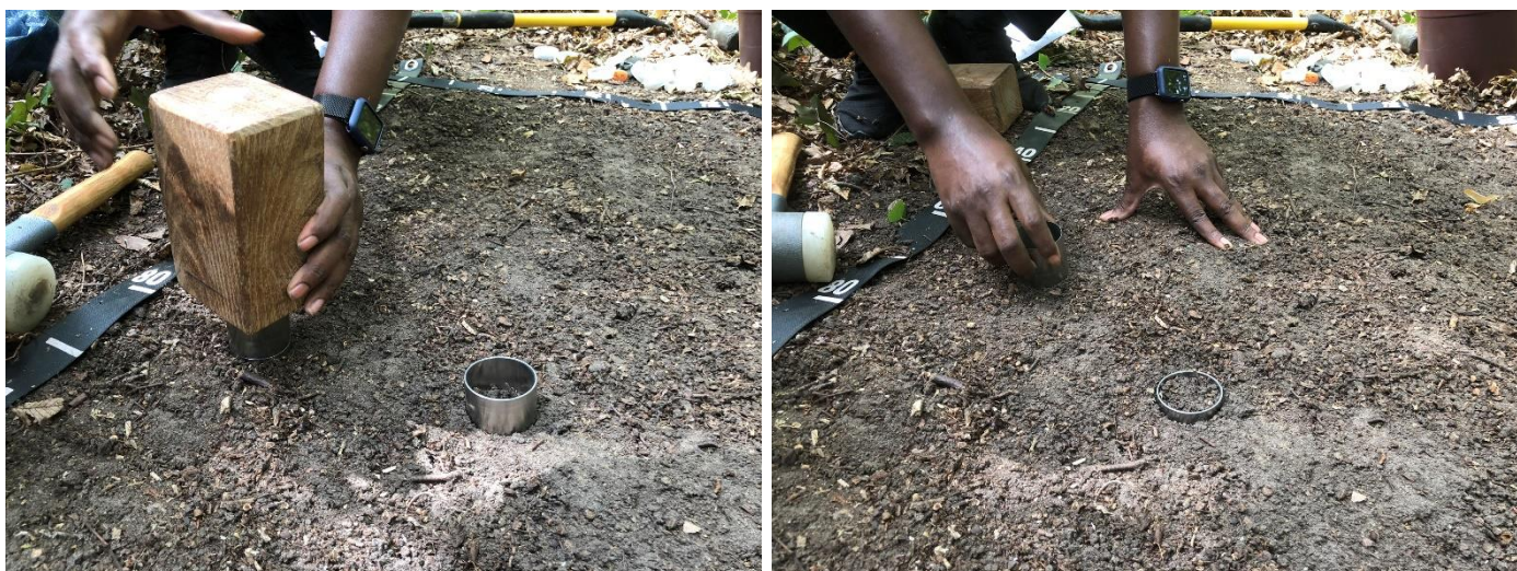
Figure 4.: The procedure of cleaning the surface and hammering the metallic ring into the soil surface
